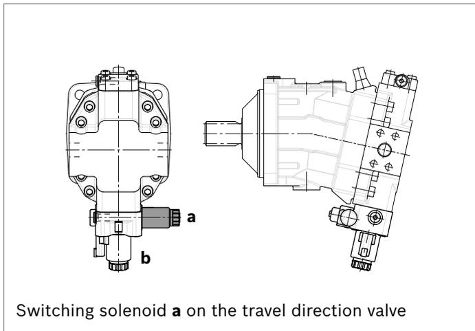
Switching solenoid a on the travel direction valve
