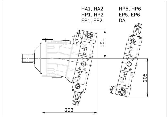
▼ **Dimensions for sizes 115 to 215 (large flushing valve)**
