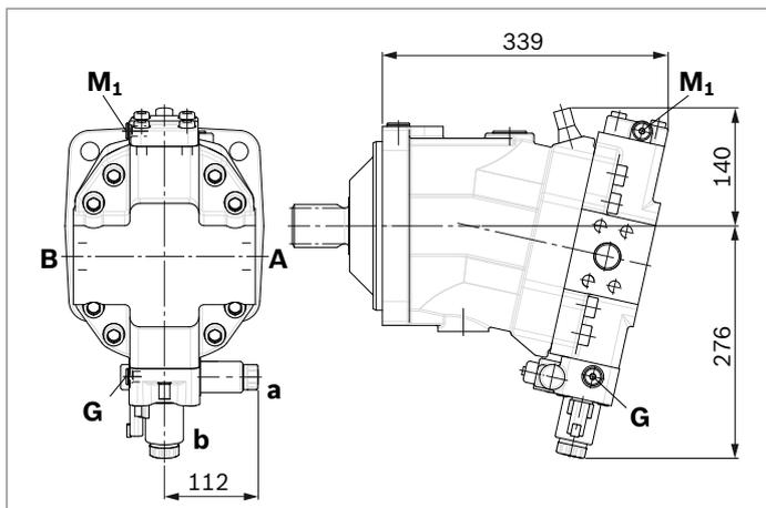
▼ **DA0** – Automatic speed-related control, negative control, with hydraulic travel direction valve
