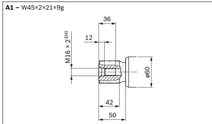
1) Involute spline acc. to ANSI B92.1a, 30° pressure angle, flat root, side fit, tolerance class 5
