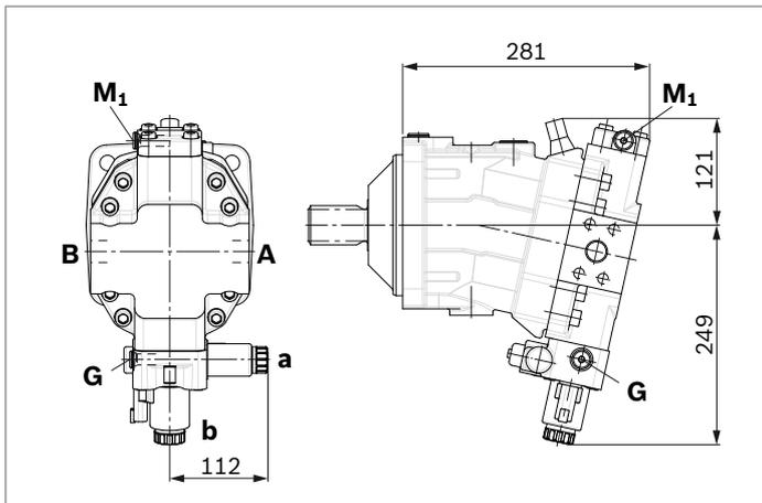
1) Port plate 1 – SAE flange ports A and B at rear
