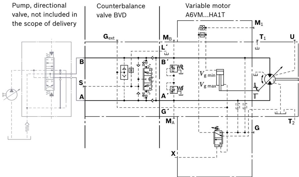
**Counterbalance valve for winches and track drives BVD...W and BVE**
