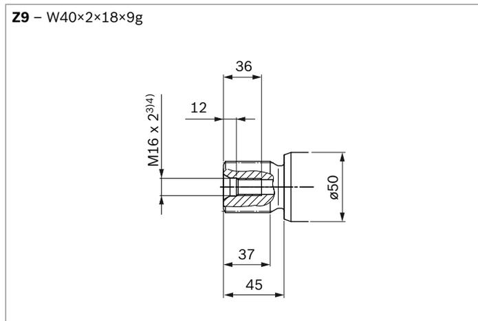
1) Involute spline acc. to ANSI B92.1a, 30° pressure angle, flat root, side fit, tolerance class 5
