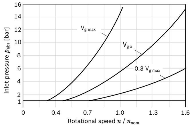
This diagram is valid only for the optimum viscosity range from  $\nu_{opt} = 36$  to  $16\text{ mm}^2/\text{s}$ .
