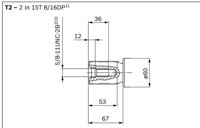
▼ **Splined shaft DIN 5480**
