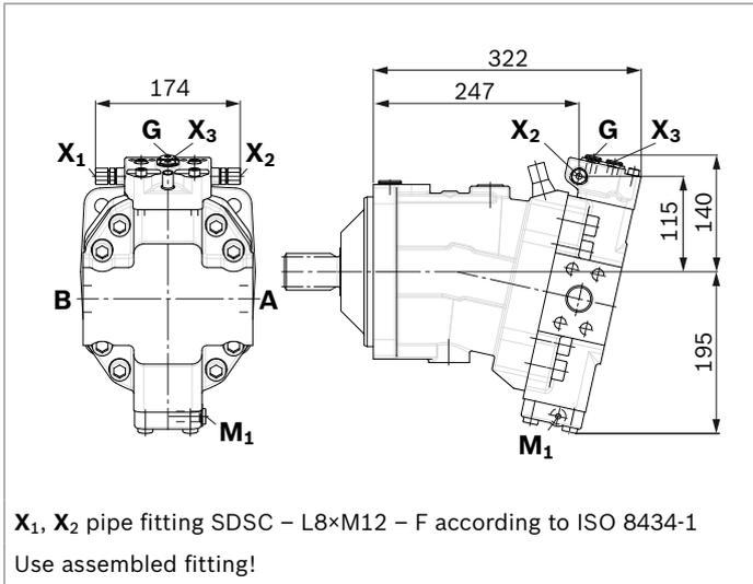
▼ **DA1, DA2** – Automatic speed-related control, negative control, with electric travel direction valve and electric  $V_{g\ max}$  circuit
