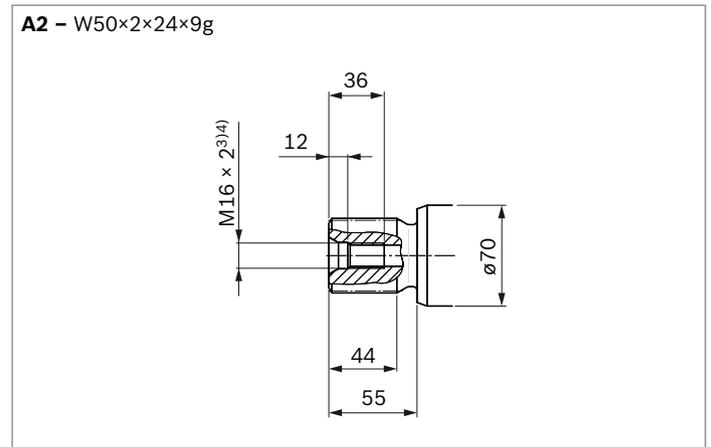
1) Involute spline acc. to ANSI B92.1a, 30° pressure angle, flat root, side fit, tolerance class 5
