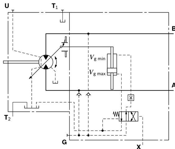
HZ7 – with throttle pin on both sides, symmetrical
