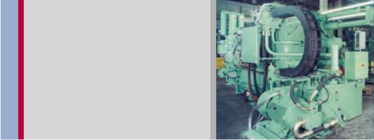
*Pressure cast machine, pump with variable pump flow thanks to drive speed control*
